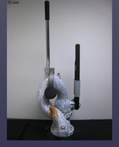
Corrosion is severe.
