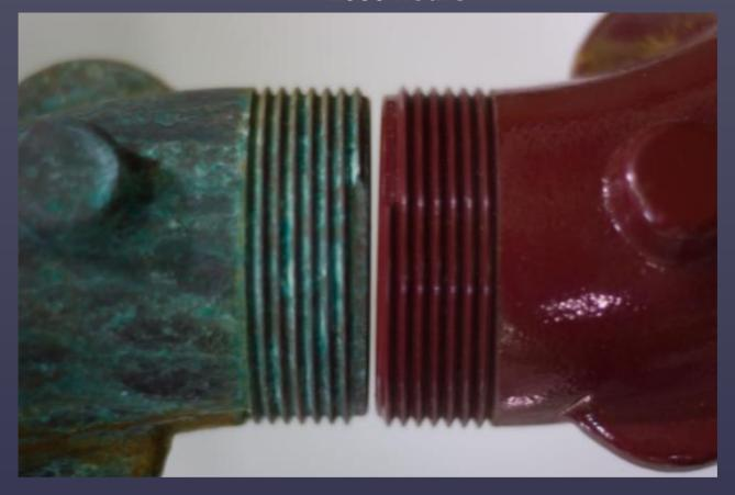
Brass corrosion builds up on threads and between moving parts.
